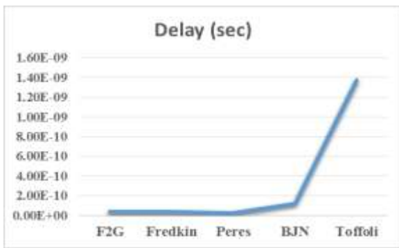
Figure 9 Delay analysis of basic reversible gates.
