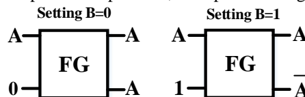
Figure 7 FG used as inverter and signal duplication.
